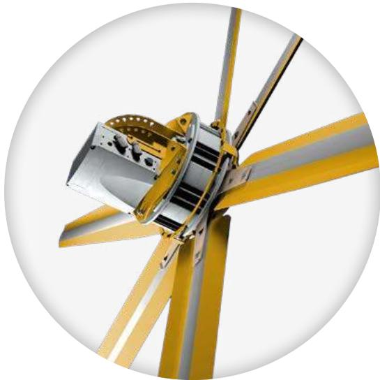
**ZEFIRO** destratifiers are the flagship of CMP. The main feature of this product is the brushless (permanent magnets) motor, which deploys an on-board mechanism for automatic and independent speed control. This innovation eliminates the gear motor located in traditional asynchronous motors, thus reducing the presence of mechanical parts subject to wear. All this results in lower maintenance requirements, greater efficiency and lower consumption.
