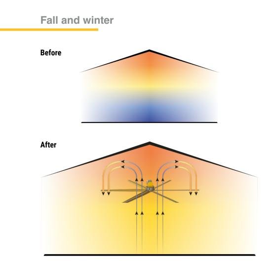
When temperature gets colder, with a simple gesture and thanks to the **Reverso** function, CMP fans mix the heat stored under the ceiling with colder air on the ground, to even out the temperature inside large rooms. Warm is directed where needed, with a consequent saving on heating costs and the improvement of people's working and living conditions.
